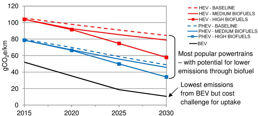
Figure 11 WTW emissions (gCO<sub>2</sub>e/km) of BEV, PHEV and HEV (segment C car, gasoline model for PHEV and HEV)
