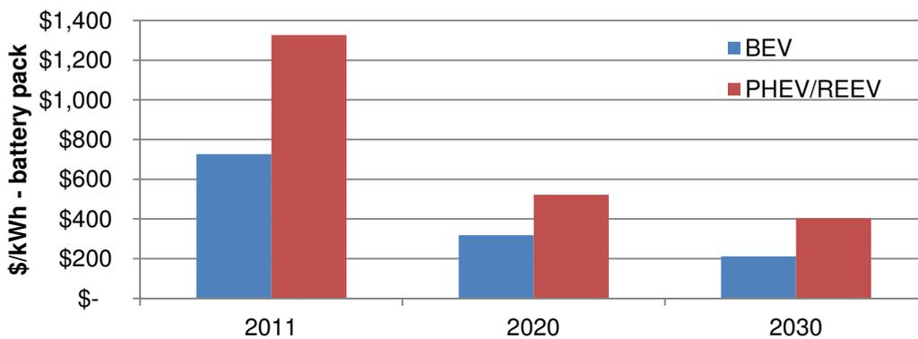
Figure 17 Battery pack cost (\$/kWh)<sup>43</sup>
